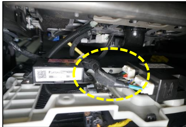
Ventilation Control Wire Harness under Front Passenger Seat
