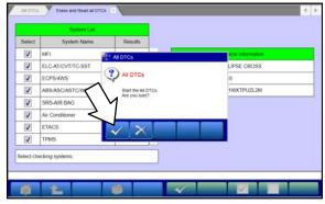
A window will pop up asking you to confirm DTC erasing. Click the check mark in the dialog box for DTC erasing and reading to begin.
