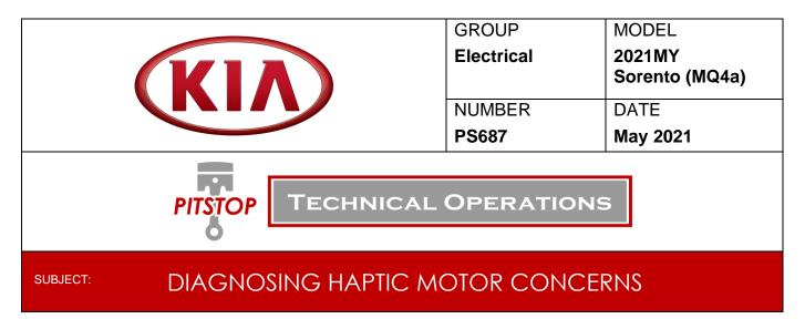
This Pitstop provides information regarding a "Check Haptic Steering Wheel System" message displayed on the cluster on some 2021MY Sorento (MQ4a) vehicles, with DTC B247300 which may be related to a poor connection in the haptic motor circuit. When diagnosing for this concern, the haptic motor circuit is shown in the 'Audio System' or 'A/V Navigation' wiring schematics and not in the steering system.
