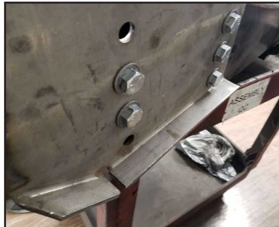
Former: Bolt with washer.
