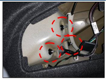
4. Carefully remove the rear combination lamp assembly.
