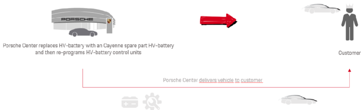
Process flow for exchange of complete battery
