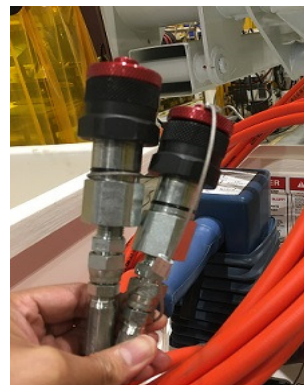
Figure 2. Bleed kit with quick couplers at boom tip
