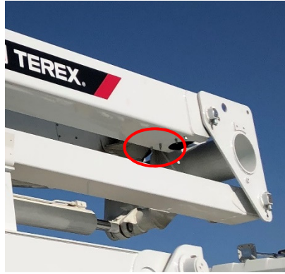
Figure 3. Elbow leveling cylinder location
