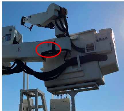
Figure 5. Boom-tip leveling cylinder location
