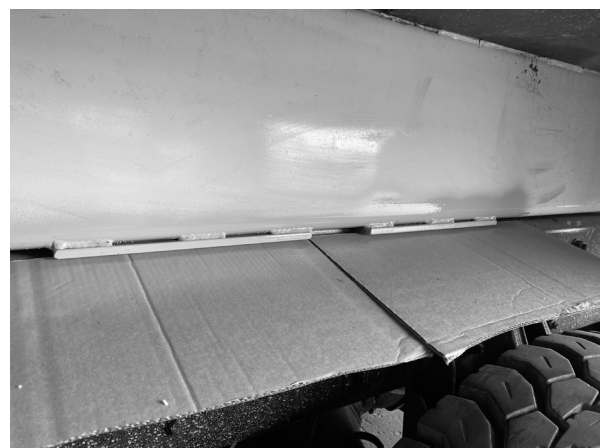
Figure 8 – Painting Repaired Areas
