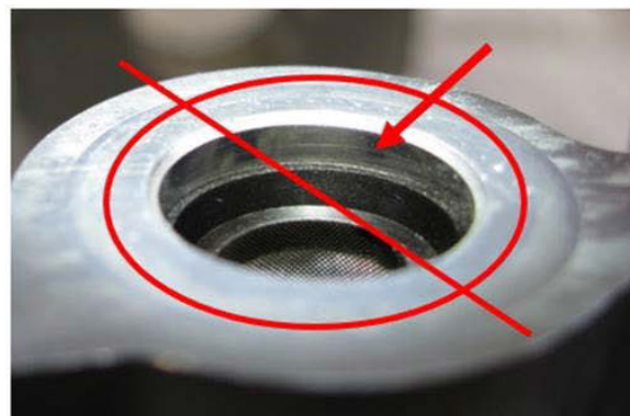
NG- Filter Screen installed too deep into the camshaft carrier bore.
