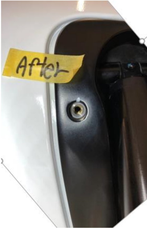
Figure 3: Airbrake panel holes aligned
