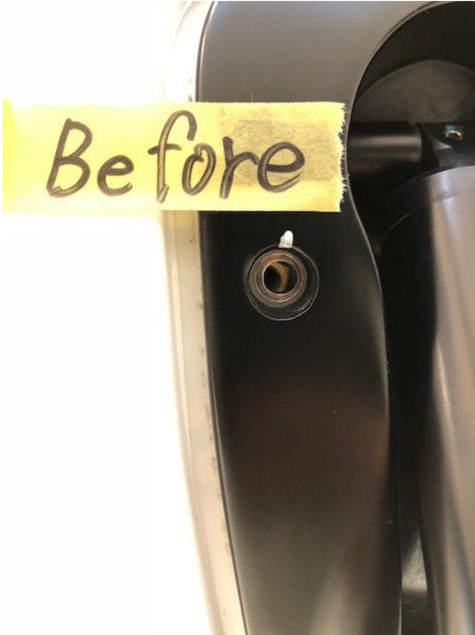
Figure 1: Airbrake panel holes not aligned.
