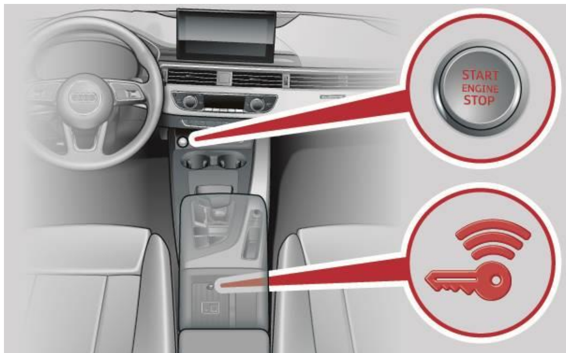
Figure 1. Center console in the Audi RS4/RS5 with a mark for the vehicle key (example).
