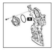
· Gaskets and pipe for high pressure fuel pump
