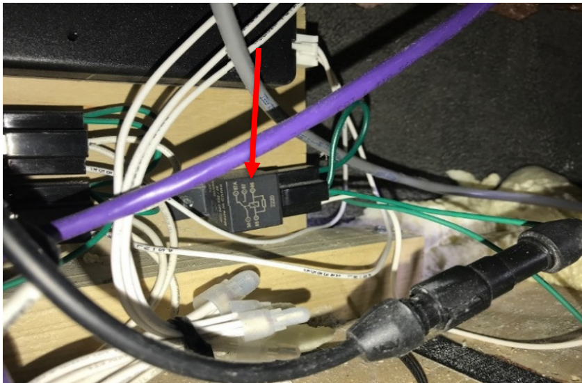
Figure 1.1 The Omnivue camera module is held against the sidewall by Velcro. Remove this module to gain access to the far-right screw holding the Trimark board in place.
