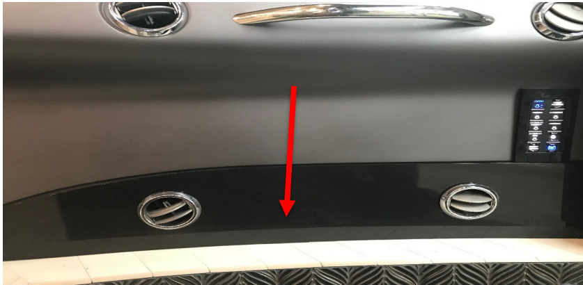
Figure 1.1 The Omnivue camera module is held against the sidewall by Velcro. Remove this module to gain access to the far-right screw holding the Trimark board in place.
