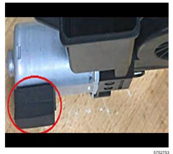
**Note:** In the graphic above, the foam is shown in the correct location on the motor housing, but will be applied to the inner door panel, not the motor housing.
