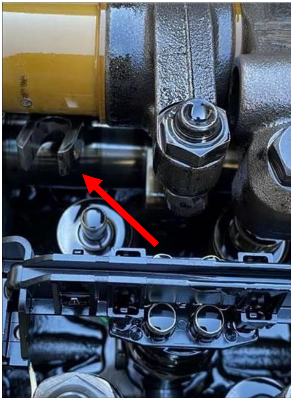
Figure 1. Exhaust Valve Bridge Out of Position
