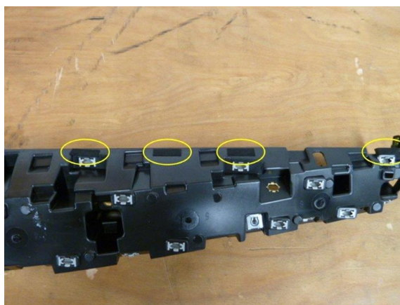
Figure 4. Apply felt strips to the circled areas.
