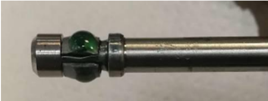
Figure 1. Locking fluid application area in the retaining pins.
