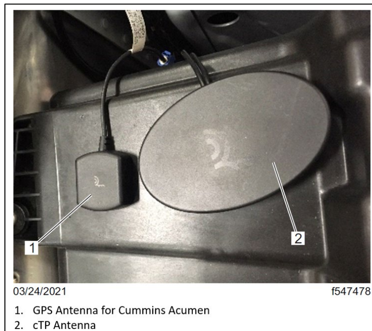
Fig. 10, GPS Antenna Mounting Location
