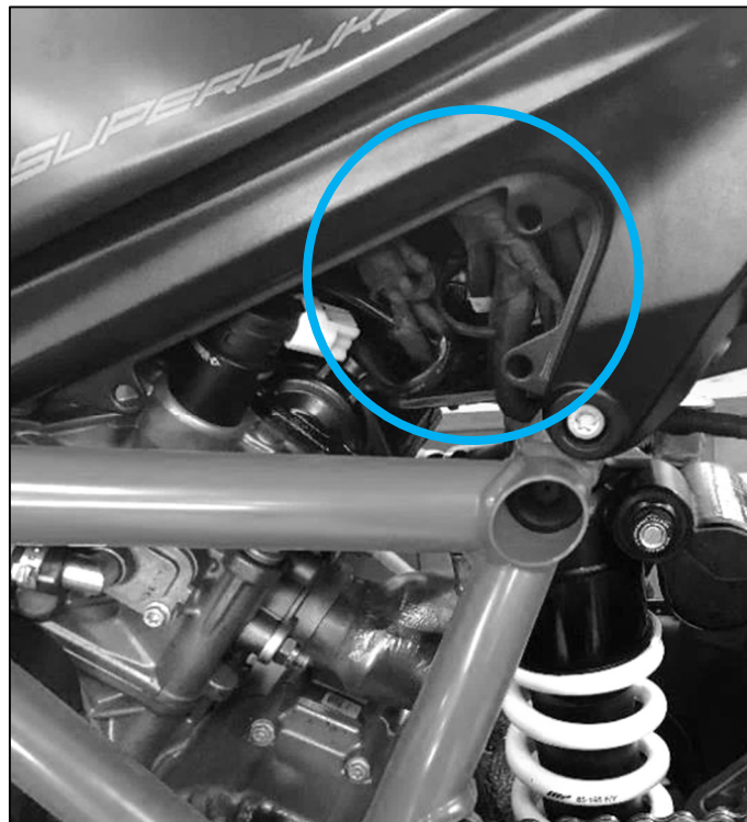
Fig. 10 - Main wiring harness area to be checked
