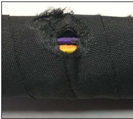
Fig. 4 - Mild or no Damage (follow code 00)
