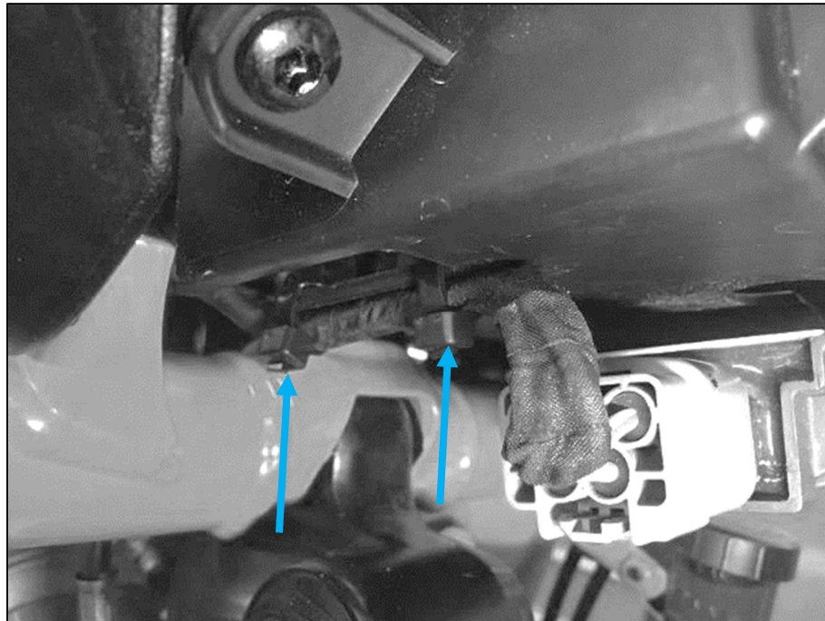
Fig. 11 - Securing the wiring harness with two cable ties
