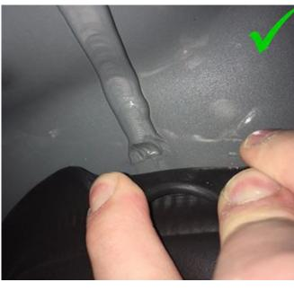
Note: Shown to the left is an example of an OK seam which doesn't require any correction.
