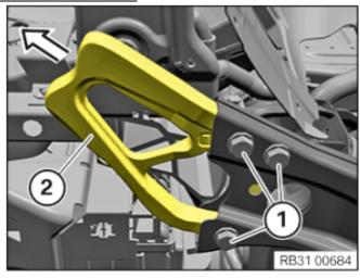
Install the left and right wedges (2) to the front axle.
