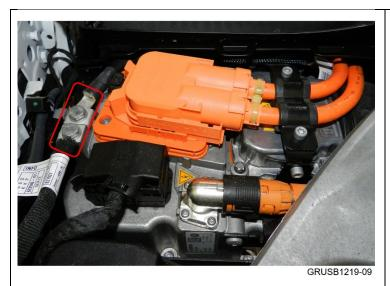
1. Remove both grounding cables at the EME. (G30 shown)
