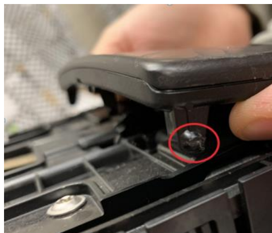
Figure 4: pin damaged due to excessive force or interference with objects inside the compartment
