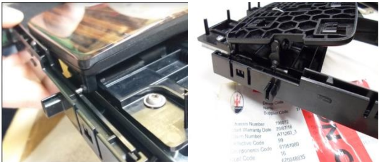
Figure 3: pins that came out of the guides caused force or interference with objects inside the compartment.
