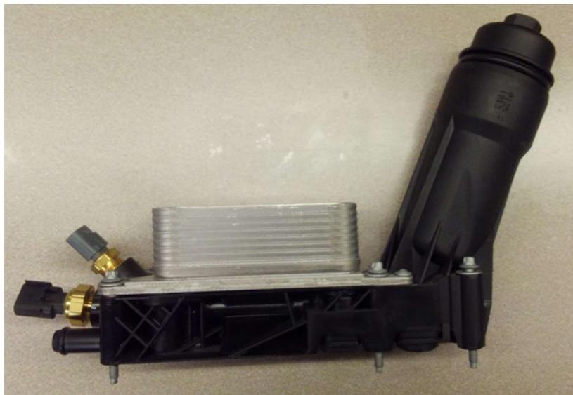
Fig 1. Oil Filter Adapter/Cooler (OFA)
