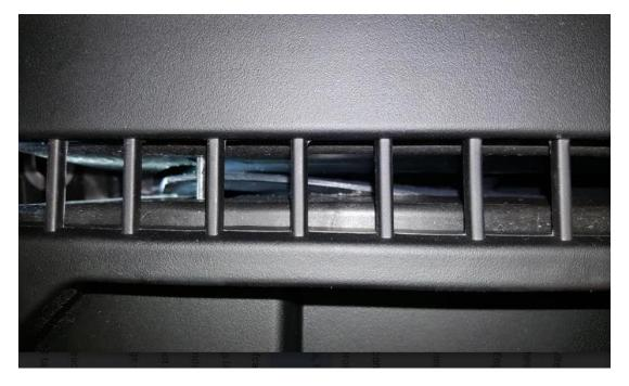
**Repair Procedure:** If this condition is found it is necessary to remove the IP cover and ensure that the defrost ducts are routed into the correct position.
