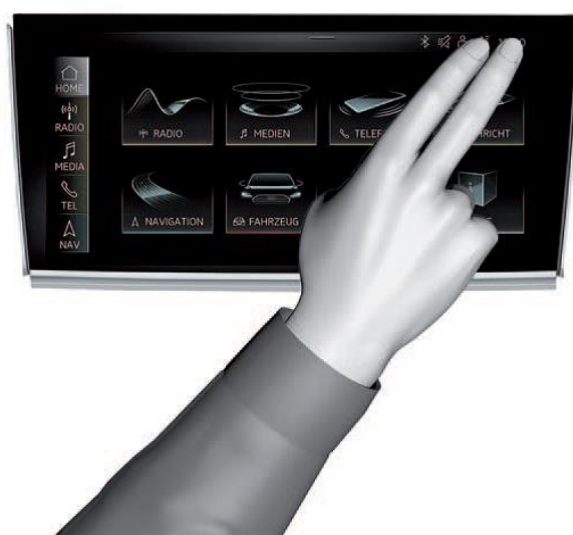
Figure 1. Gesture to enter the red engineering menu.
