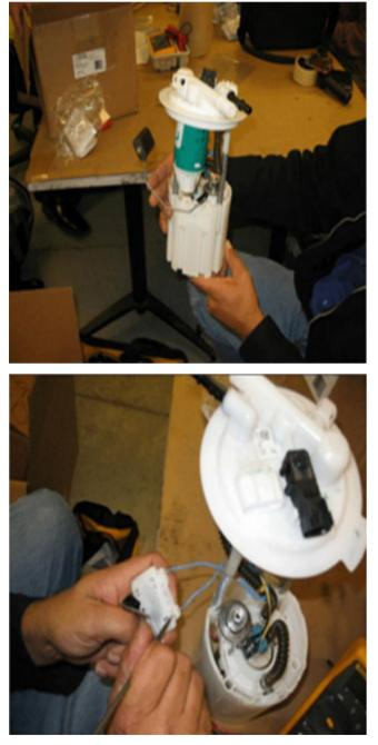
Once sensor is removed from assembly carefully depress lock tabs on both sides of the sensor to remove the terminals from the fuel level sensor assembly. Install terminals into a new fuel level sensor.
