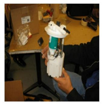
Upon a successful sweep test, reinstall module into the fuel tank, reassemble the components and verify successful repair.
