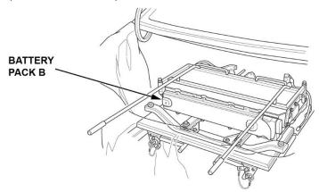
44. If needed, flip the battery pack upside-down, and remove the IPU center frame.
