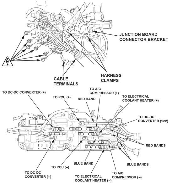
19. Disconnect the right lower IPU harness connector and remove the junction board connector bracket.
