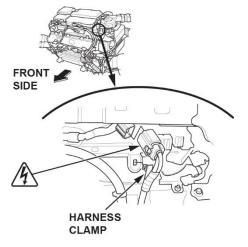
8. Remove the harness clamp, then disconnect the D/V 12 volt plus cable and the ground cable.
