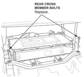
40. Place fender covers over the rear fenders and the trunk opening to avoid damaging the vehicle. Attach the battery removal/installation carrier onto battery pack. Loosely tighten the bolts. Install the carrier adapter mount with the "B" mark side to right rear battery pack mount. Loosely tighten the bolts then tighten the five bolts to **24.4 N·m (18 lb·ft)**.
