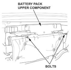
18. Battery Pack A removal: From the cabin side, disconnect the high voltage motor power inverter module cable terminals and remove the harness clamps, then remove the junction board connector bracket.
