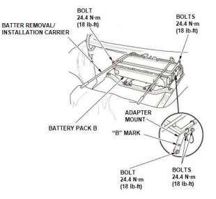
41. Install the inside handle to the battery removal/installation carrier and install the pin. Set the battery removal/installation table in the trunk area as shown (table legs folded).
