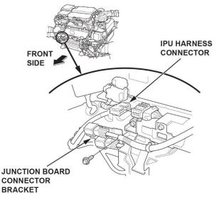
20. Disconnect the battery system leak sensor connector and remove the junction board.
