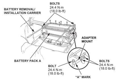
30. Install the inside handle to the battery removal/installation carrier and install the pin. Set the battery removal/installation table in the trunk area with the table legs extended.
