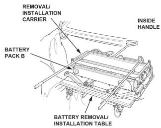
43. With the help of an assistant at the rear of the vehicle, carefully lift the battery pack B and remove it from the trunk area. Set the battery pack on the work surface provided with the Accord PHEV Battery R&R Equipment Loan Kit (07PHEVBATOLKIT).
