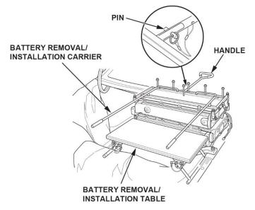
31. With the help of an assistant on the inside of the vehicle, carefully lift and transfer battery pack A onto the battery removal/installation table. Remove the inside handle from the battery pack removal/installation carrier.
