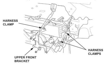
26. From the trunk side, disconnect the left IPU lower harness connector.
