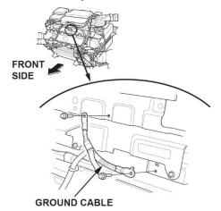
7. Disconnect the high voltage motor power inverter module cable connector and remove the harness clamp.
