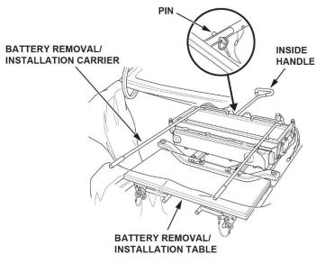
42. With the help of an assistant on the inside of the vehicle, carefully lift and transfer battery pack B onto the battery removal/installation table. Remove the inside handle from the battery pack removal/installation carrier.
