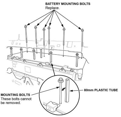
29. Place fender covers over the rear fenders and the trunk opening to avoid damaging the vehicle. Attach the battery removal/installation carrier onto battery pack A. Loosely tighten the bolts. Install the carrier adapter mount with the "A" mark side to the right rear battery pack mount. Loosely tighten the bolts, then tighten the five bolts to 24.4 N·m (18 lb·ft)
