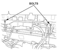
17. From the trunk side remove the bolts, then carefully remove the battery pack upper component from the trunk.
