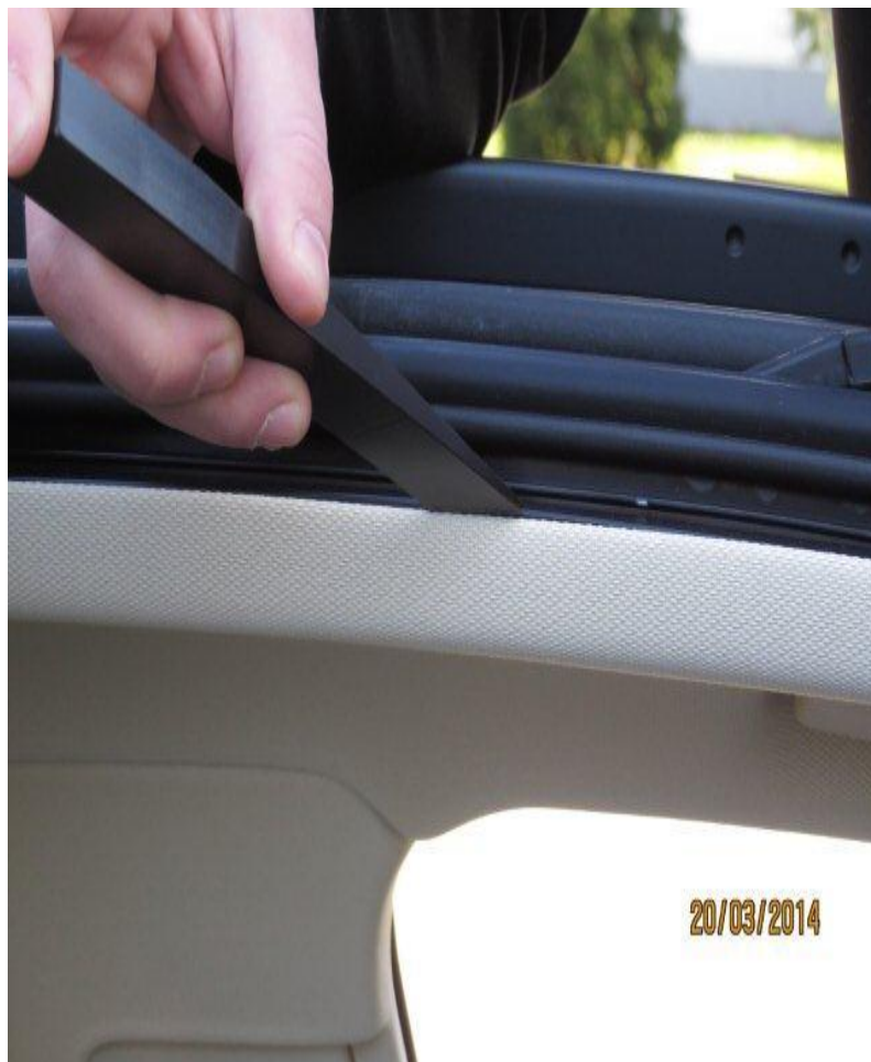
Figure 1. Unclipping the sunroof cover trim frame.
