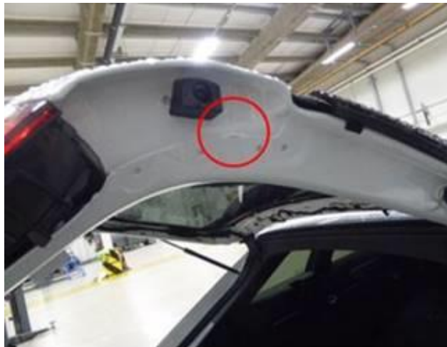
Figure 6. Sealer flaw on side of rear lid.
