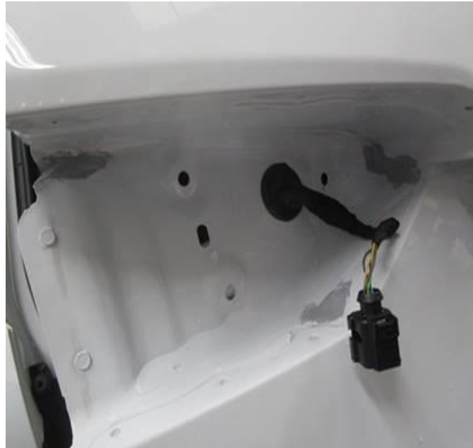
Figure 9. Concealed areas repaired with D 511 500 A2 1k adhesive sealant.
