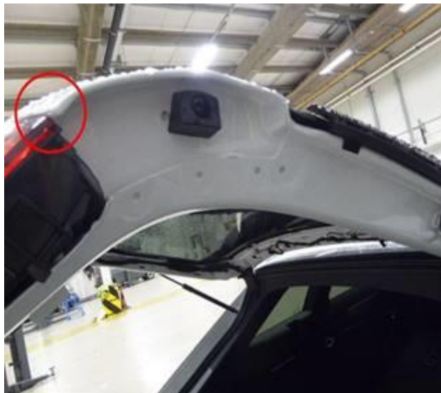
Figure 2. Area where sealer flaw is likely.
