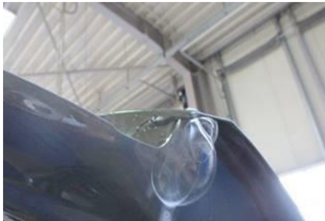
Figure 1. Bubble formation with compressed air applied internally.
