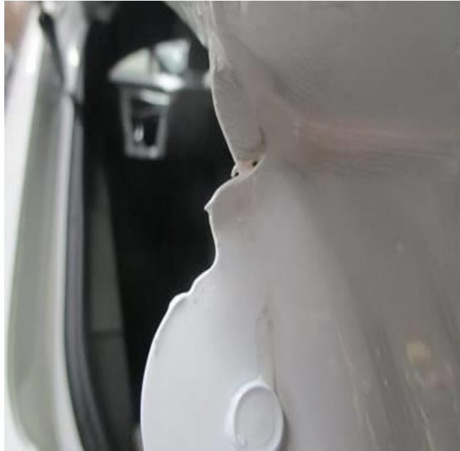
Figure 3. Possible sealer flaw area behind tail lamp.
