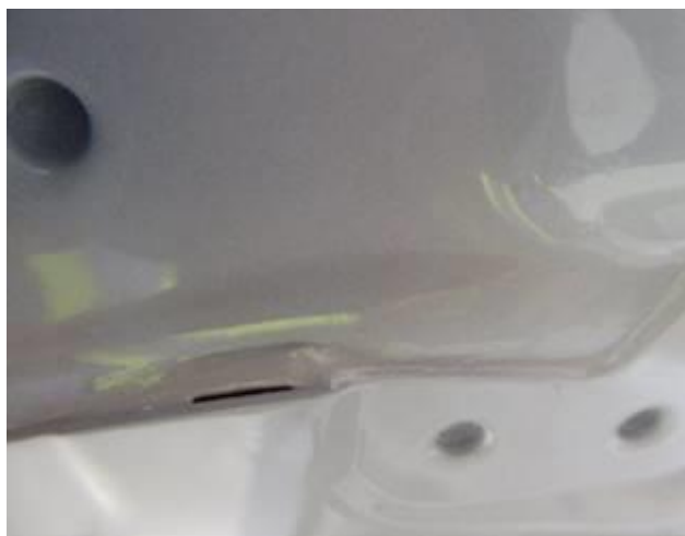
Figure 7. Close up view of the sealer flaw.
