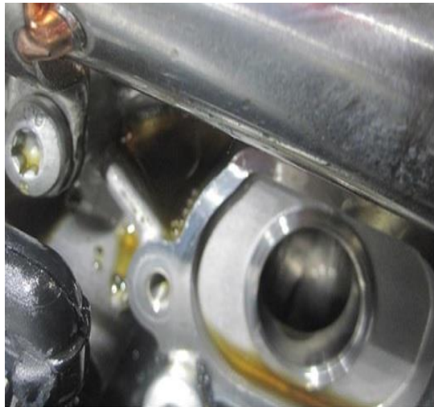
Figure 2. Oil in the Audi valve lift system.
