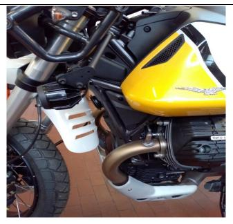
Remove the left hand guard of the headstock, P/N 2B005529.
