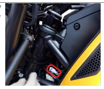
Move the connector into the correct position and secure it to the connector of the regulator with a cable tie.
