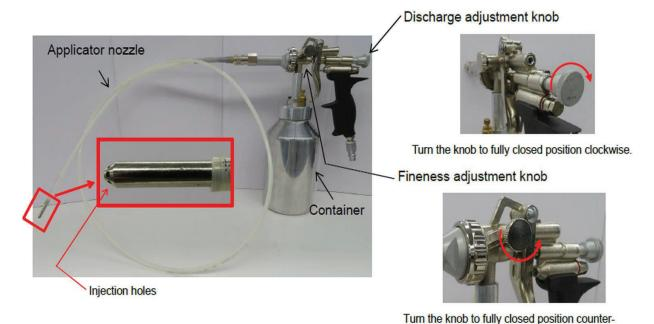
c. Remove the cap on the gun container and fill with anti-corrosion agent.
