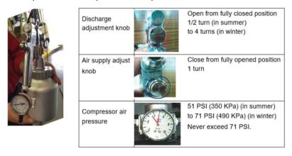
g. Test the spray gun by fully engaging the gun trigger to confirm anti-corrosion agent is injected from nozzle.
