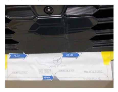
7. Position the Bracket onto the Bumper, locate the center hole and insert **provided** Self-Tapping Screw at the previously placed mark. Tighten partially to complete step #8.
