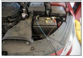
15. Connect the SST power cables to a fully charged 12V battery or to an external AC/DC power supply.
