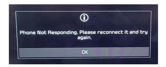
NOTE 1: If the intermittent Wireless CarPlay disconnection occurred, do not replace the radio. The disconnection phenomenon is caused by the Apple IOS software. Apple IOS software intermittently pause the data transmission, causing the communication interruption between the radio and CarPlay.
