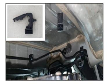
7b. Note the white alignment marks on the brake tubes coincide with the holders in some locations.
