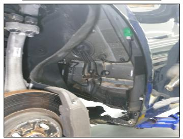
4. Remove the vehicle under covers as shown (front driver's side, and rear left and right covers).
