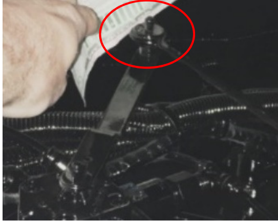
Figure 2. Top end of ride height control linkage
