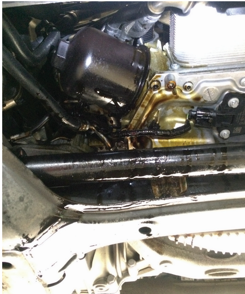
Active leak #1 Overview of the engine showing an active oil leak with oil droplets forming.
