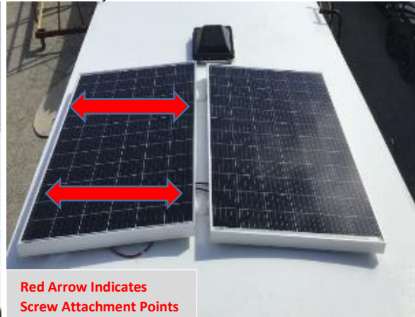
FIG - 2 Primary Solar Panel – Screw Removal Points
