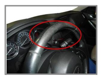
**NOTE:**Slight wear on a seam of the steering wheel is not applicable to this bulletin. It is inevitable since friction and force are applied while turning the steering wheel.
