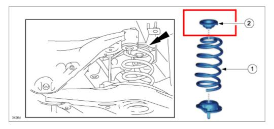
8. Install the rear coil spring with the spring oriented as shown below.
