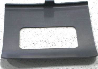
G37407 TEMPLATE USED TO CUT DASHBOARD COVER FOR HUD INSTALLATION
