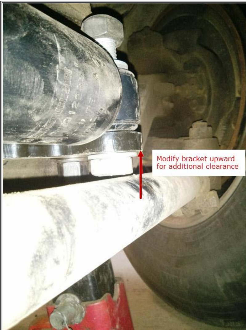
Figure 4: Tie rod tube to mount clearance
