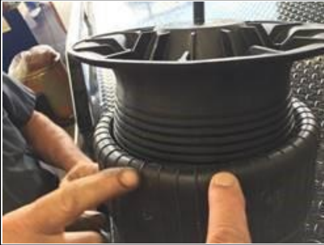
Figure 4: Torn Air Spring
