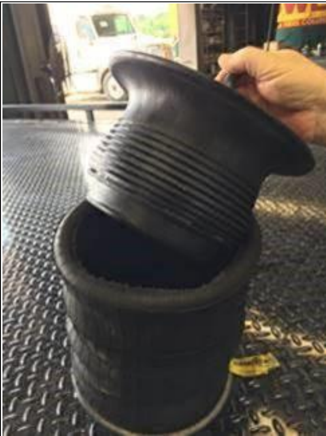
Figure 5: Damaged Air Spring
