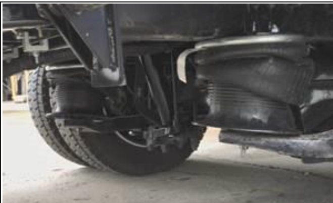
Figure 3: Pinched Suspension Air Spring (CONDITION IS NOT NORMAL)
