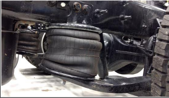
Figure 1: Normal view of air spring when suspension is dumped
