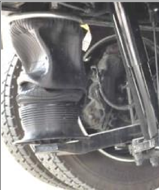
Figure 2: Collapsed Suspension Air Spring
