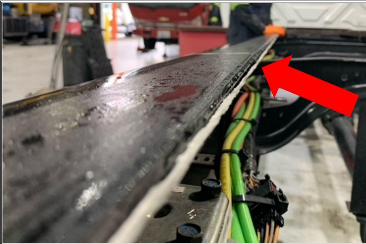
Figure 4: Example of String Test on a Rail with a Center Bulge
