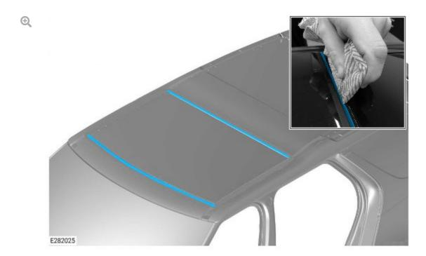
Insert the tool and cloth between the glass roof panel flip seal and the vehicle body.
