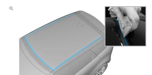
Insert the tool and cloth between the glass roof panel flip seal and the vehicle body.
