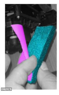
Remove the protective backing from 1 adhesive foam pad.
