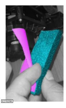
Remove the protective backing from the other adhesive foam pad.
