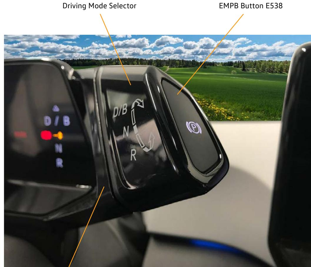
Steering Column Switch Module with J527
