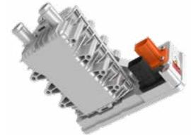
**ZX17** High-Voltage Heater (PTC) is a cabin air heater and contains both the high-voltage heater (PTC) Z115 and the control module. It has an output of up to 6,000 watts and can be regulated in three stages.
