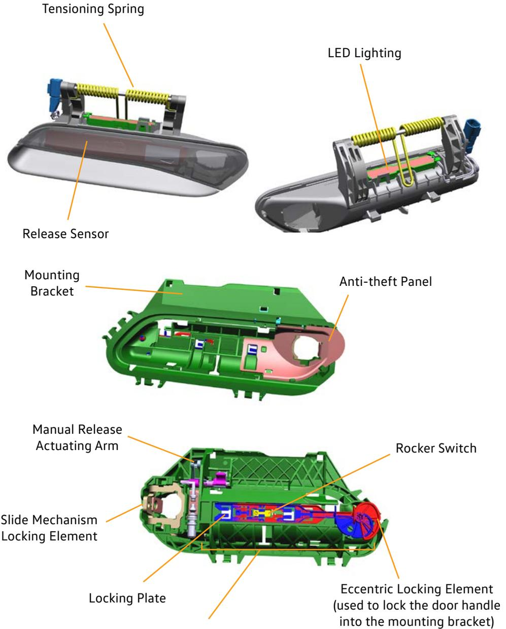
Red indicates the starting position of the handle locking assembly.
