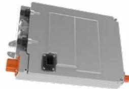
**JX1** Power and Control Electronics for Electric Drive converts the customer's power requests into electrical signals. The power electronics control the three-phase current drive. DC voltage from the high-voltage battery is converted into a three-phase AC voltage for acceleration.
