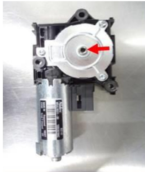
Figure 3. Sunroof motor V1 or sunroof sunshade motor V260.
